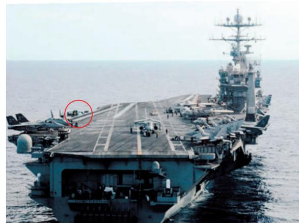
An Improved Fresnel Lens Optical Landing System unit isn't all about the meatball. “Wave-off” lights flash if the deck is not ready for a landing. Coming in too low? “Cut” lights mean, strangely, add power.
