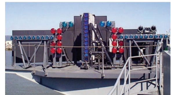
With a low, six-foot profile, the IFLOLS unit allows wings loaded with fuel, sensors, and armament to easily pass overhead on takeoff.
